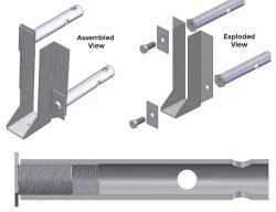
Double threaded cylinder bolt assembled
