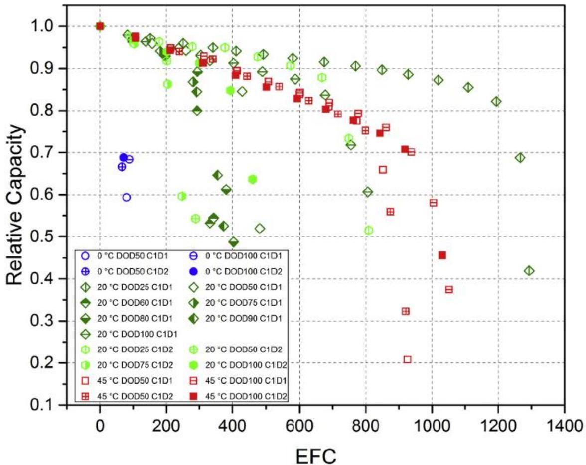
Lithium batteries lose their capacity as they age. Both Lithium and Lead Acid batteries lose cycles at higher temperatures. Assuming 20C temperature and 50% DoD, Lithium capacity will drop between 0.5% and 1.5% per month. Suggesting 8 to 12 year life span when used.
